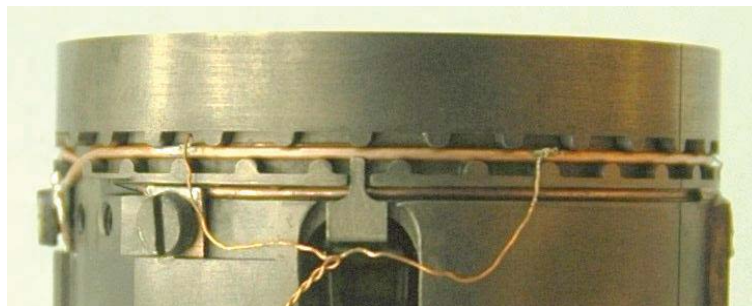
Figure 5-14. Position of the voltage taps in the TARSIS bending test.
